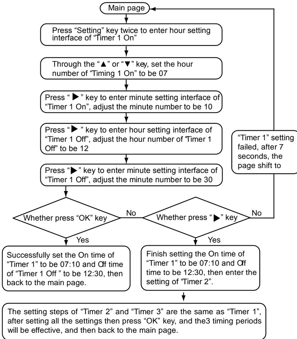
During any period of timing setting to press "OK" key , then the timing period has been set will be effective (only when the "On" and "Off" of one timing period have been set then this period setting can be finished).
