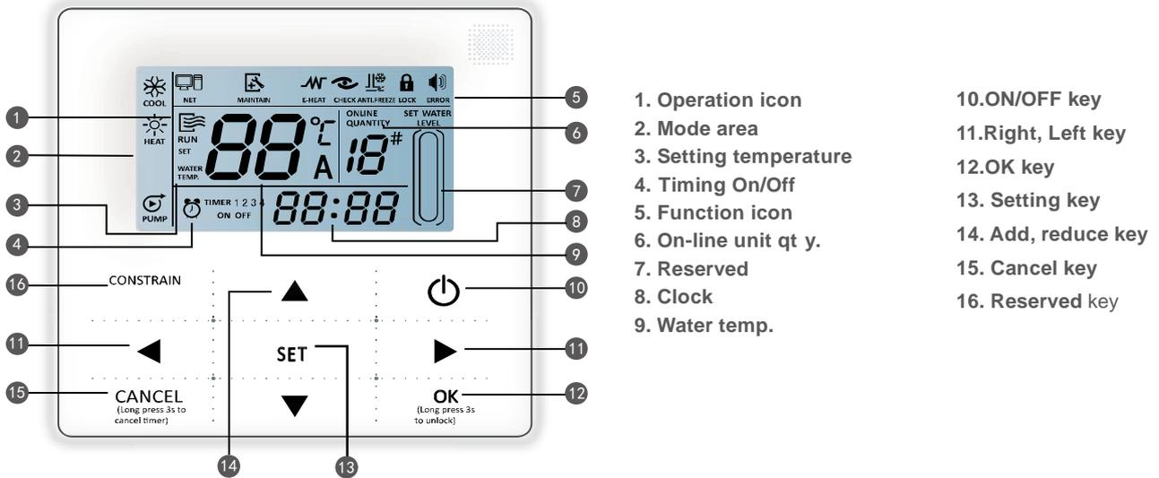
①. **Operation icon** : Indicate the ON and OFF status; when it is ON, it will display; when it is OFF, it will disappear;
