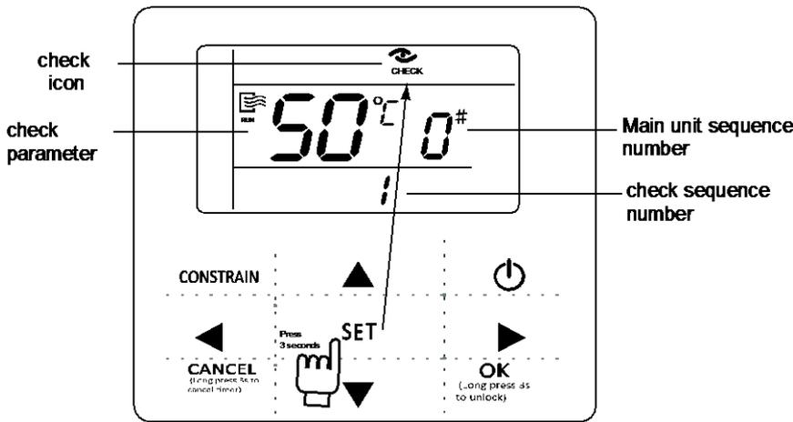
3) Press the “▲” or “▼” key to adjust the main unit serial number can query 16 sets main units status information from #0~#15. Press “◀” or “▶” to adjust the spot check sequence number of one main unit then can query all the status information of this unit. Spot check content according to the main unit model wired controller :
