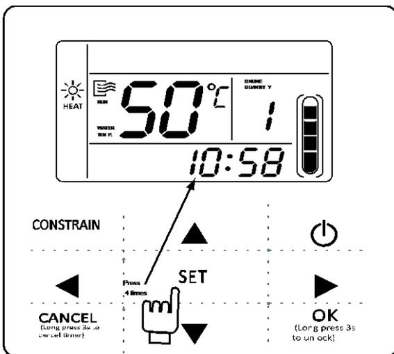
▲ This time the hour of the clock will flash, it means the current setting is the hour of the clock, press the “▲” or “▼” to adjust, press “▶” key when finished, and then the minute of the clock will flash, it means the current setting is the minute of the clock, press the “▲” or “▼” to adjust, press “OK” key when finished or wait for 7 seconds to be effective; during the setting process press the “Cancel” key, then it will exit without saving.
