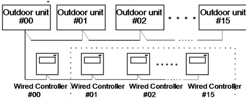
Use PQE connect with each other when several wired-controllers are parallel.
