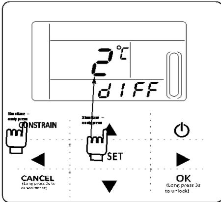
Operation method: Turned off, press the "Constrain" "▲" 2 button for 3 seconds to enter the hysteresis setting selection. Can be adjusted Hysteresis parameter  $\delta = (2,3,4,5 \text{ } ^\circ \text{C})$ . Press "◀" or "▶" key to select the desired value, 7S key operation Or press the Enter key, then exit and save the settings and return to the main page. During setup, press the "Cancel" key, does not save the parameters and exit.
