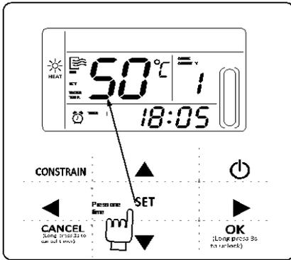
Query water temperature setting: press the “◀” or “▶” key under the main page to query the set water temperature numerical value.
