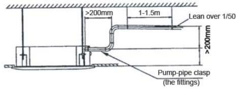
■ The end of the drainpipe should be over 50mm higher than the ground or the bottom of the drainage chute, and do not immerse it in water. If you discharge the water directly into sewage is sure to make a U-form aqua seal by bending the pipe up to prevent the smelly gas entering the house through the drain pipe.
