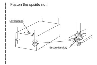
• Install the hanging bolt into U groove of the hanging tool. Overhang the indoor unit and ensure it is level using a level gauge.
