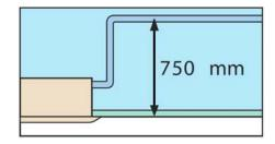
After upward piping, the lead drain pipe must slant downward immediately. (Over 1/100)
