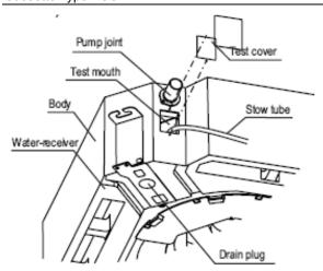
2. Turn on the power, and operate the air conditioner under the "COOLING" mode. Listen to the sound of the drain pump. Check whether the water is discharged well (a lag of 1min is allowed before discharging, according to the length of the drain pipe), and check whether water leaks from the joints.
