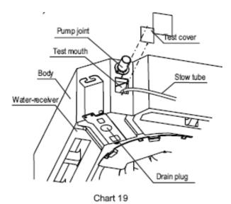
2. Turn on the power, and operate the air conditioner under the "COOLING" mode. Listen to the sound of the drain pump. Check whether the water is discharged well (a lag of 1min is allowed before discharging, according to the length of the drain pipe), and check whether water leaks from the joints.
