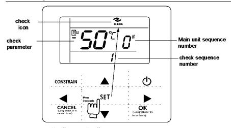
3) Press the "▲" or "▼" key to adjust the main unit serial number can query 16 sets main units status information from #0∼#15. Press "◄" or "▶" to adjust the spot check sequence number of one main unit then can query all the status information of this unit. Spot check content according to the main unit model wired controller:
