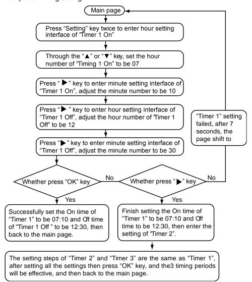
During any period of timing setting to press "OK" key, then the timing period has been set will be effective (only when the "On" and "Off" of one timing period have been set then this period setting can be finished). Press "Cancel" then cancel the setting. Query timing information: if query the timing hour which has been set, press "◀" or "▶" key under main page, the On and Off time of Timer1, Timer 2 and Timer 3 will be displayed in turns.
