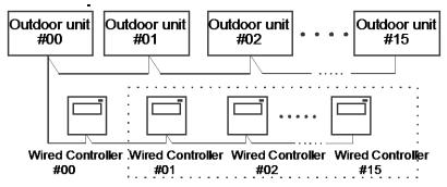
Use PQE connect with each other when several wired-controllers are parallel.
