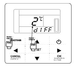
Operation method: Turned off, press the "Constrain" " $\blacktriangle$ " 2 button for 3 seconds to enter the hysteresis setting selection. Can be adjusted Hysteresis parameter  $\delta = (2,3,4,5\,^{\circ}$  C). Press " $\blacktriangleleft$ " or " $\blacktriangleright$ " key to select the desired value, 7S key operation Or press the Enter key, then exit and save the settings and return to the main page. During setup, press the "Cancel" key, does not save the parameters and exit.
